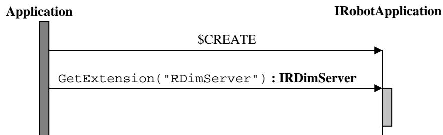
Having gained the access to the RDIM module server, which is the **IRDimServer** interface, an external application is able – by obtaining the relevant interface – to carry out all the operations needed by calculations:
