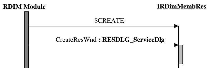
MVCS component has the indicator to the RdimConnection interface (it has been passed by means of the Connect method of the IRDimClient interface), using which it may communicate with RDIM module calling up appropriate methods. In this way it may also acquire indispensable instances of some interfaces.
