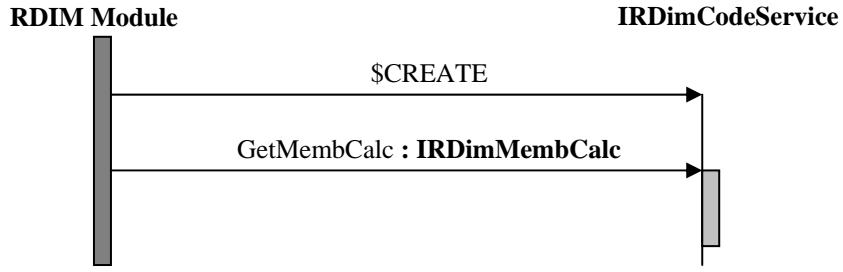
Having obtained the object of the IRDimMembCalc interface, RDIM module may carry out any calculations of member verification, group verification or design. It sets input parameters at any calculation point by means of the following:
