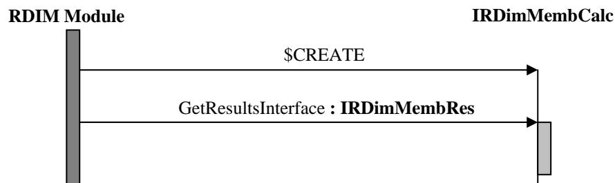
From the interface acquired by means of this method standard calculation results are taken. Access to specific, typically code-dependent numeric results is gained by RDIM module by calling up the CodeResults method.
