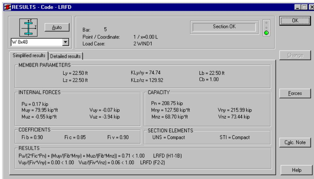
There is the 'Calculation Note' button provided in the above dialog box, which when pressed generates a calculation note in an RTF file format. A calculation note is generated based on a template whose variables are replaced with the relevant values. RDIM module employs the IRDimMembRes interface for this purpose, activating appropriate methods sequentially. These are:
