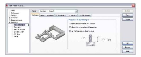
On the Model tab of the Object Inspector, right-click Building, and click Create foundation plan or, click ASD Drawings ➤ Drawings
