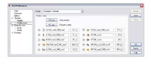
**NOTE** The Job Preferences dialog lets you define the syntax of names assigned to positions created during automatic positioning of structure elements. After the syntax for an arbitrary structure element is defined, the field to the right of the syntax displays a preview of an element name resulting from the defined syntax.
