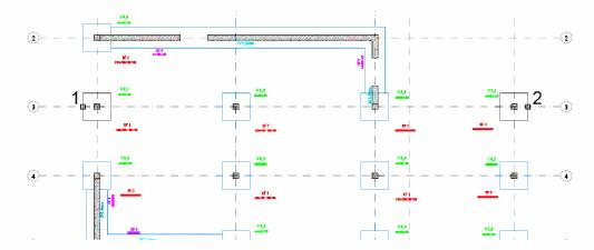
**NOTE** The software draws the dimension line for the indicated elements, and will group dimension lines appropriately.
