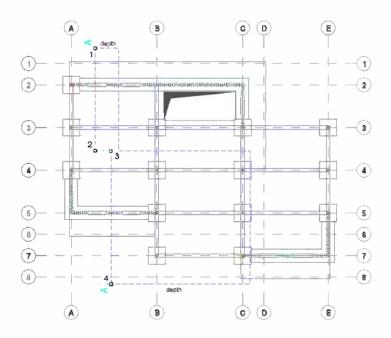
2 Click ASD Drawings ➤ Drawings Edition ➤ (Insert elevation mark). Alternatively, click Formwork Drawings menu ➤ Insert elevation mark. Insert elevation marks as shown below. Just click once to add elevation mark.
