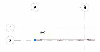
■ Using the same method, define windows in the walls on axes 5 and 7 as shown.
