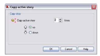
**NOTE** Higher stories were created automatically. Notice that not all of the selected elements were copied. Elements characteristic only for the ground-floor level (such as footings) were omitted.
