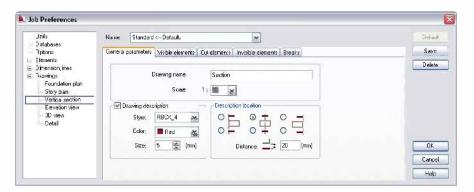
**NOTE** After you have finished editing a structure model, you can indicate the location where you want to create a vertical section of the model.
