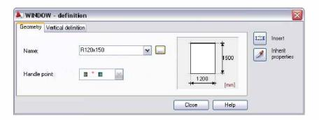
On the Vertical definition tab, specify the level of the window with respect to wall as **600**, and then click (Insert) to insert the selected window type.
