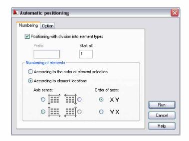
**NOTE** Positioning gives names to elements (assigns an identifier or position), and detects all identical and differing elements in individual groups. It also counts the total number of identical elements in individual positions. The operation of automatically assigning a position is possible for a whole structure model or for a selected part (a story or an element type, for example).
