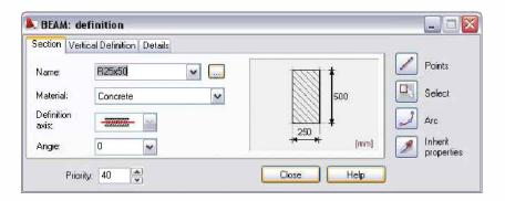
**NOTE** You can quickly create round or rectangular sections by specifying required parameters for Name. An acceptable syntax for a round section is D250 (diameter) and for a rectangular section is R200x400 (width x height).
