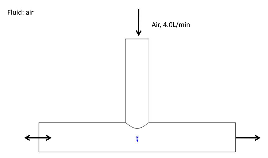
Air, transient flow (similar to a piston pushing and pulling air)
