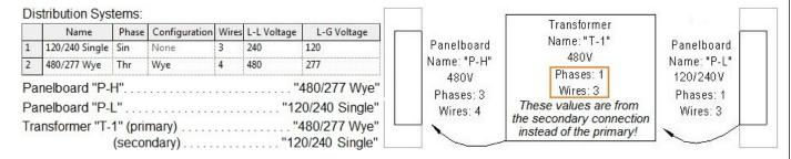
**Work-Around:** Create a dedicated Electrical Equipment Tag for transformers that either displays a static text value or reports Shared Parameters in lieu of reporting the actual "Number of Phases" and "Number of Wires" parameters.
