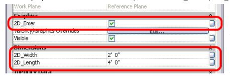
Again, click the tiny button on the right hand side of the emergency fill parameter and create a new parameter in the light fixture family to link it too. This should be a type parameter since
