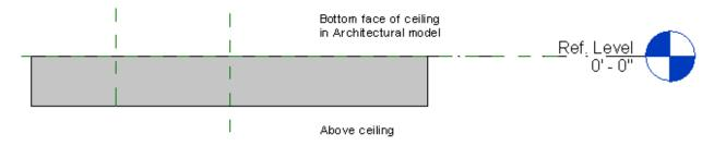
Draw a reference plane *below* Ref. Level to represent the *top* surface of the fixture. Dimension and label this plane also.
