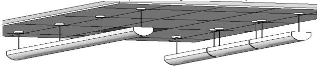
the right hand side of the image, simply creating a 4 ft. fixture and copying it for the desired total length. This however does not match the way that the lighting fixture will actually be installed. To begin with, the manufacturer provides wiring for a single point of power for any of the available lengths. The example on the right would have an electrical connector for each of
