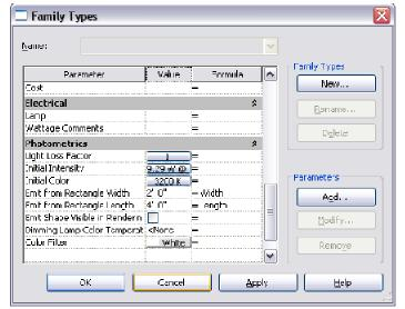
Parameters for setting the light source width and length. Use the formula field to make these parameters equal to the Width and Length that drive the dimensions we placed earlier.
