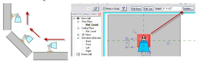
The next issue that must be resolved is the visibility of the geometry and the plan view symbol. For fixtures like these, typical practice is to show a scalable symbol on your plan view representing a wall sconce. This means that we must hide the geometry in the family in the appropriate view orientation. Because we are rotating the entire family to a vertical wall surface, the Plan/RCP view
