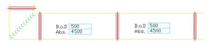
**Example - Pipe work -** Reporting Levels from Elevation Datum (Finished Floor Level) to Centre Line
