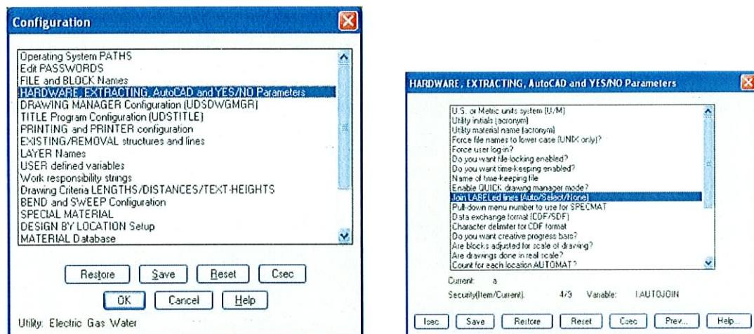
Select: **HARDWARE, EXTRACTING, AutoCAD and YES/NO Parameters** (double click)
