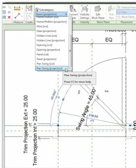
Figure 10: All symbol lines in plan to be of subcategory Plan Swing (projection).
