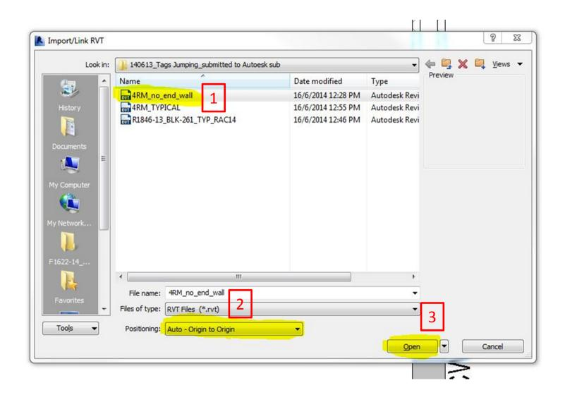
STEP 4. After linking the 4RM-no\_end\_wall to the file, go to Visibility/Graphic Overrides, Revit Links tab, then select By Host View. From the RVT Link Display Settings, Basic Tab, select the By linked view button. Select Floor Plan: Base level\_annotation\_CHECK from the Linked View, then OK.
