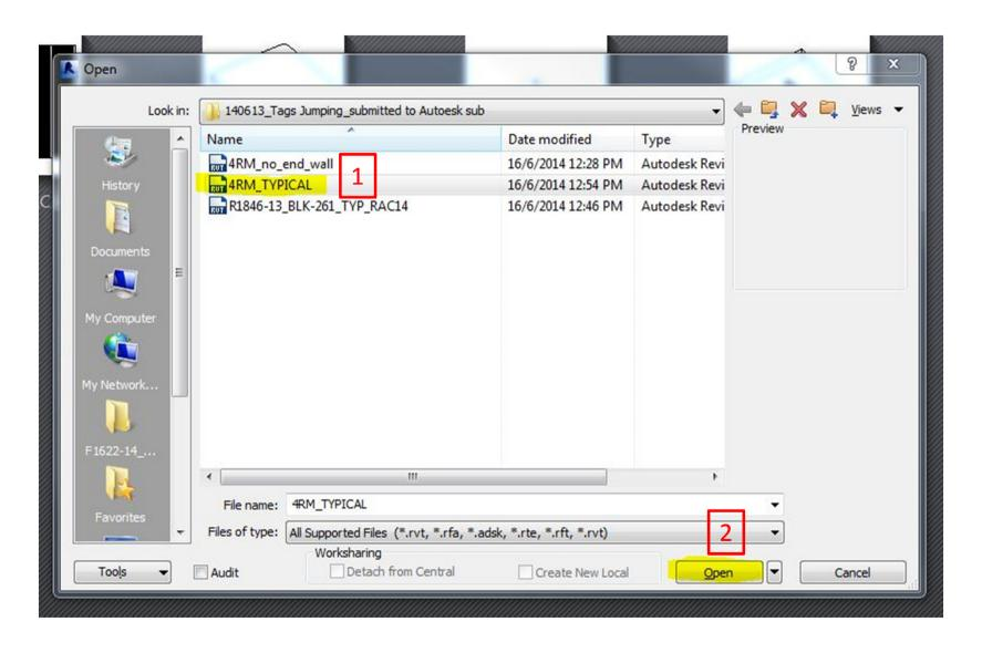
STEP 3. After opening the 4RM\_TYPICAL file, go to Import/Link RVT, link 4RM\_no\_end\_wall file using the positioning Auto-Origin to Origin then Open.
