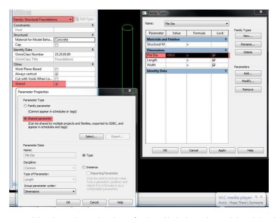
I nested the Pile Family into the Pile Cap family and locked it in place and shared the Pile Dia parameter. This family Shared box was also ticked. I placed Formula in this family so that when I change the Pile Diameter all the pile cap parameters change to suit. The centers of the Piles change but the pile diameter stays the same. I have to change that separately. Surely there is something that I have missed. I wish to change the Pile Dia parameter once and it change everything.
