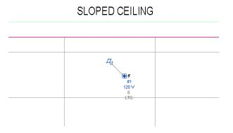
For this reason it is recommended that an arrow is placed in the family to match the slope direction. Draw the arrow using model lines with the <Invisible Lines> subcategory. This will prevent the arrow from showing up in sections. It will only appear when hovering over the fixture. You can also apply the visibility parameter called "Plan Symbol Visibility".
