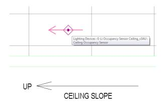
Next add a parameter called "Plan Symbol Visibility". This parameter will be yes/no parameter and have a formula driven by the "Plan Symbol Slope" so that if there is no slope, only 1 will appear. Apply this parameter to the "Lighting Device 1" that is placed on the "Left", "Right", and "Back" planes. When placed this fixture on a sloped ceiling, Revit will not show the 3 symbols that are not parallel to the floor.
