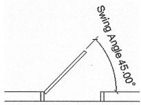
Link this dimension to a parameter called swing angle. This parameter should be an Instance as each door may vary depending on location or phase. It may be grouped under the Dimensions or Graphics headers.
